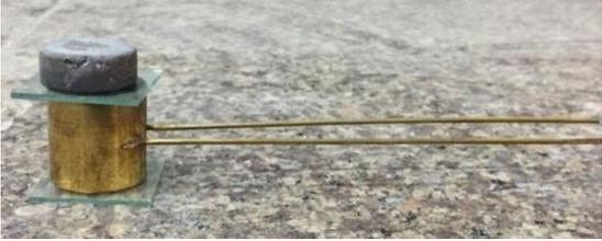
A photograph of a Le Chatlier apparatus, which consists of a cylindrical brass container with a green base and a dark, cylindrical weight on top. A thin metal rod is attached to the side of the container. |
