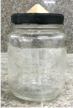
A photograph of a glass pycnometer, which is a laboratory instrument used for measuring the density of solids. It consists of a glass jar with a stopper and a small funnel on top.                        |
